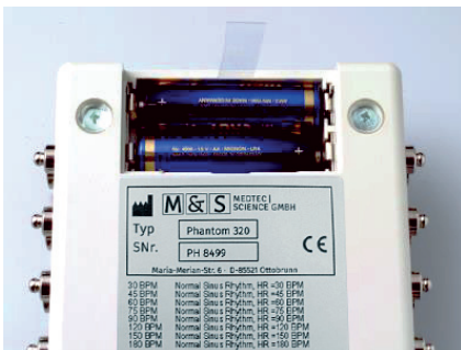
Figure 7-1: Battery compartment of the phantom 320
